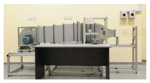
Figure 4. Small, open-loop, subsonic wind tunnel of the NUS Temasek Laboratories.
