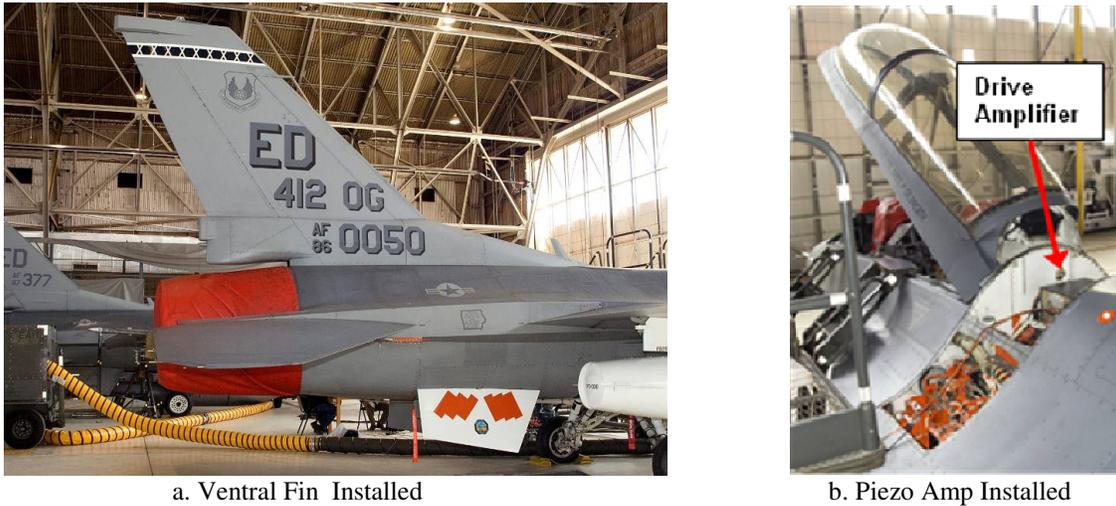
Figure 17. ACTIVE FIN Installed on Test Aircraft. (photos courtesy of Edwards AFB, PA)
