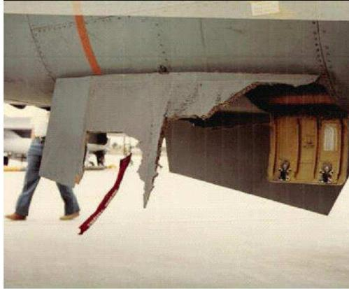
Figure 2. F-16 Block-15 Ventral Fin Failure Example.
