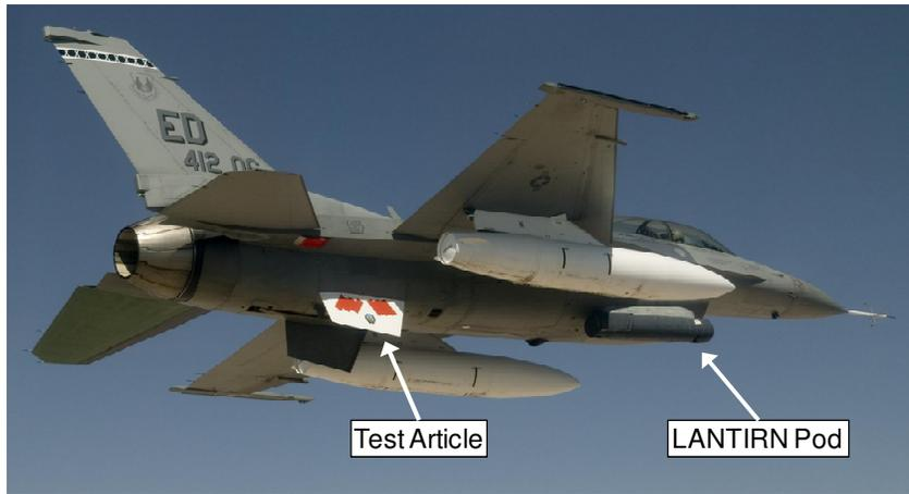
Figure 21. ACTIVE FIN Instrumented Test Aircraft. (photos courtesy of Edwards AFB, PA)
