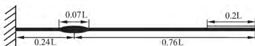
Figure 7. Optimized MFC-magnet energy harvester mechanical structure.
