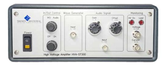
Two independent signal inputs are provided — a wave generator input and an audio signal input — both of which are selected by a rotary switches. The wave generator input accepts signals in the range of 0V to +10V at a frequency of 0 Hz to 1 kHz. The audio signal input accepts audio signals in the range of 0 to 10 V at a frequency of 0 Hz to 1 kHz. Two potentiometers are also provided to adjust the gain and the offset of the audio signal.
