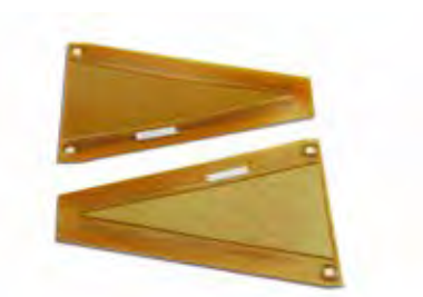
triangular MFC for strain adaptation
