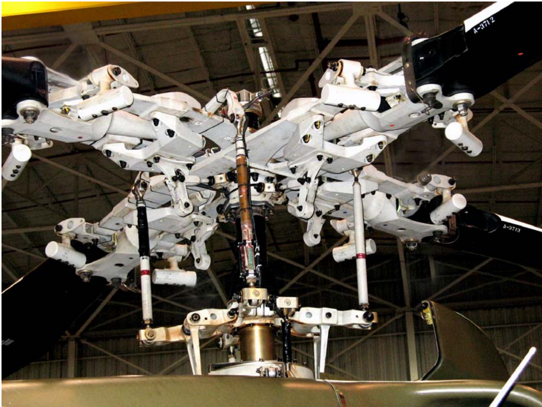
Figure 8. Energy harvesting wireless pitch link installed on Bell M412
