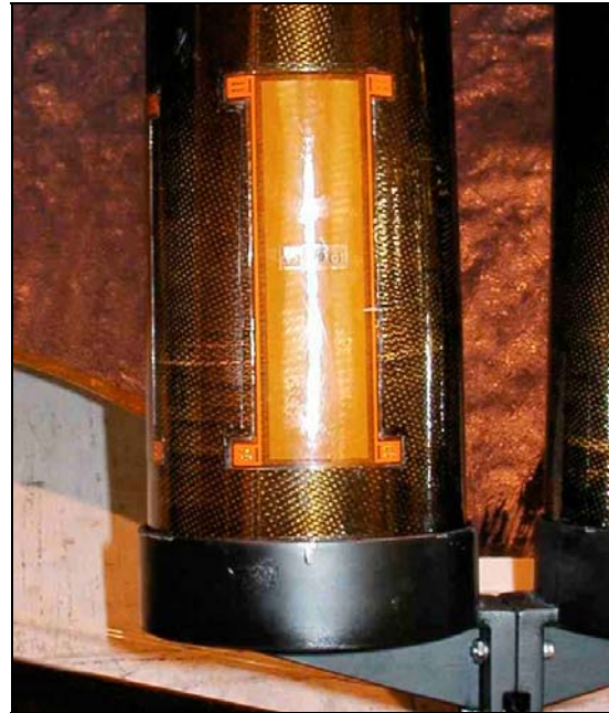
Figure 7. LaRC MFC Actuator Installed on Tapered Tube
